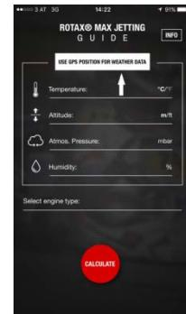
2. As a second step, the engine type of the kart needs to be selected. Therefore the button underneath the weather data needs to be clicked. The App will automatically show all potential Max evo engines from which one can be selected by clicking on a certain engine type.
